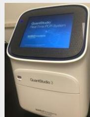
**Figure 5. Photo of QuantStudio 3.** QuantStudio 3 was the machine used to perform qRT-PCR reaction and measure fluorescence signals from SYBR green.
